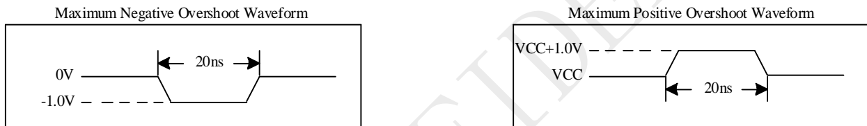
Figure 5-2 Input Test Waveforms and Measurement Level
